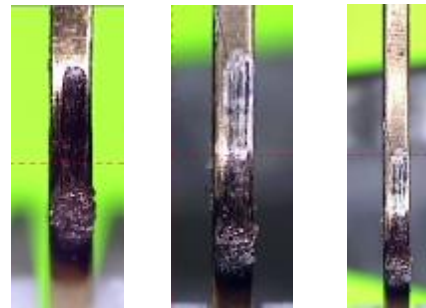
Variations in socket contact design and resulting damage
