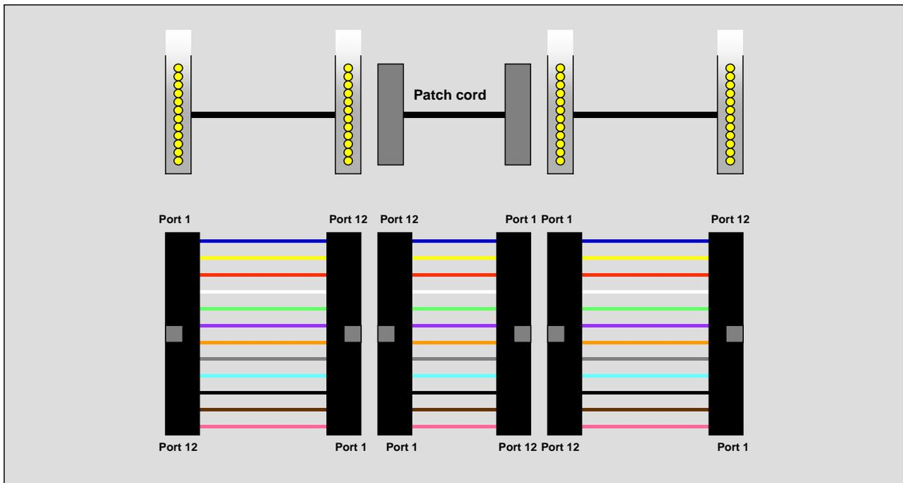
Figure A.1 - Optical fibre polarity within channels containing fixed cabling with array interfaces
