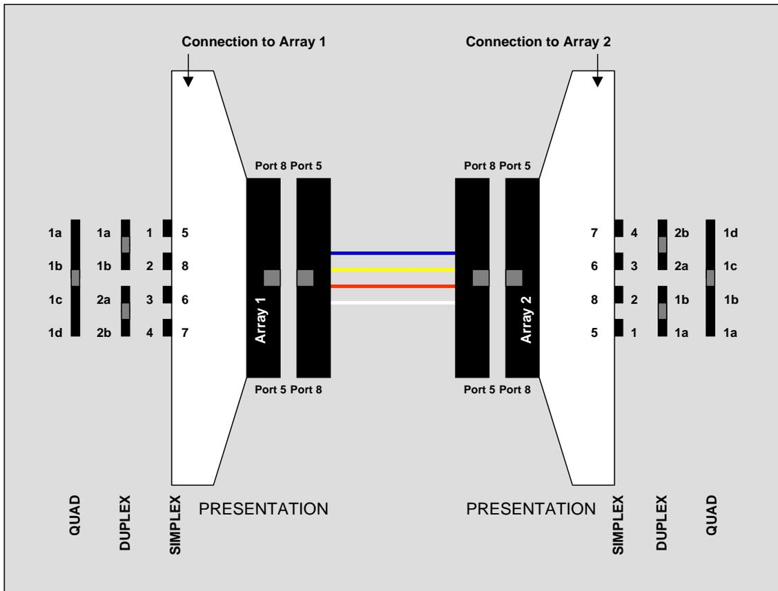
Figure A.4: 4-element presentations of a 12-element array pre-terminated interface
