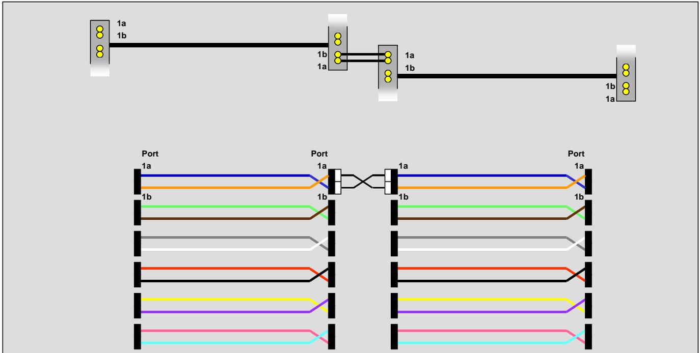
Figure 3: Optical fibre polarity within channels containing fixed cabling with duplex interfaces
