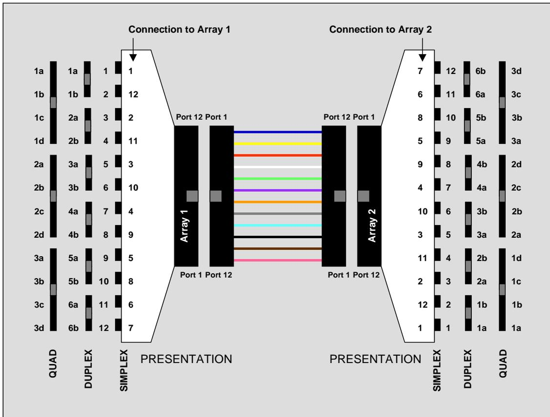
Figure A.2: 12-element presentations of a 12-element array pre-terminated interface
