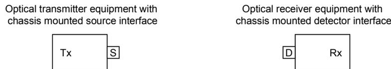
Figure 2: Transmission equipment convention
