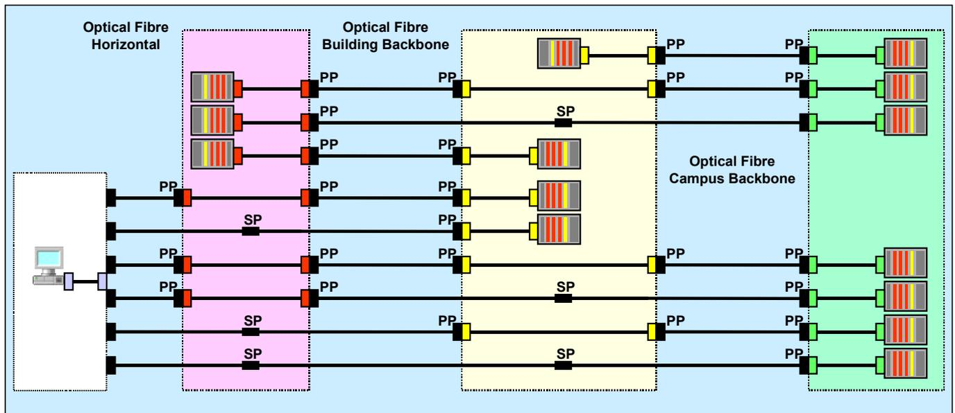
Figure 7: Typical configurations of optical fibre cabling within premises
