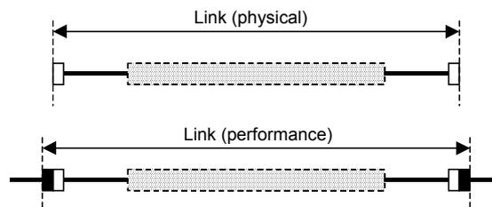
Figure 4: Optical fibre links - physical and performance
