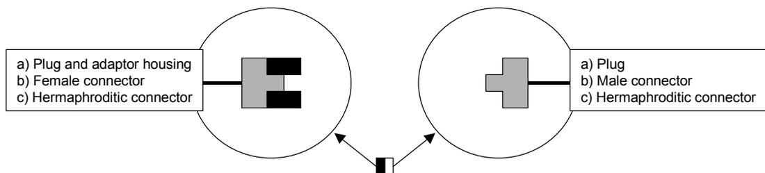
Figure 1: Connecting hardware convention
