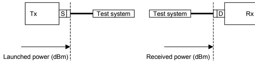
Figure 5: Launched and received power reference points
