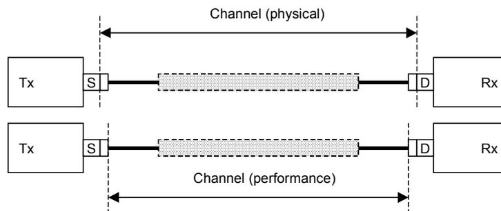
Figure 3: Optical fibre channel - physical and performance
