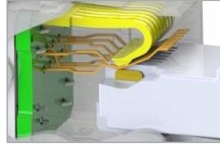
Plug fully engaged in connector
