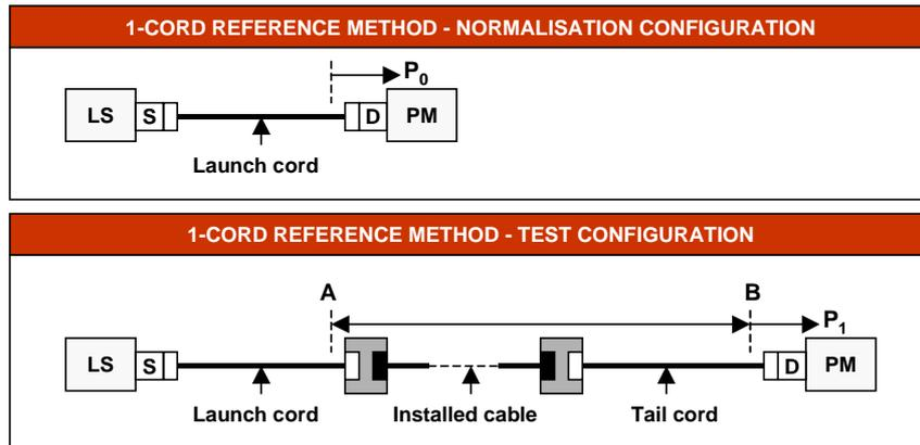
Figure 4 - 1-Cord Reference testing
