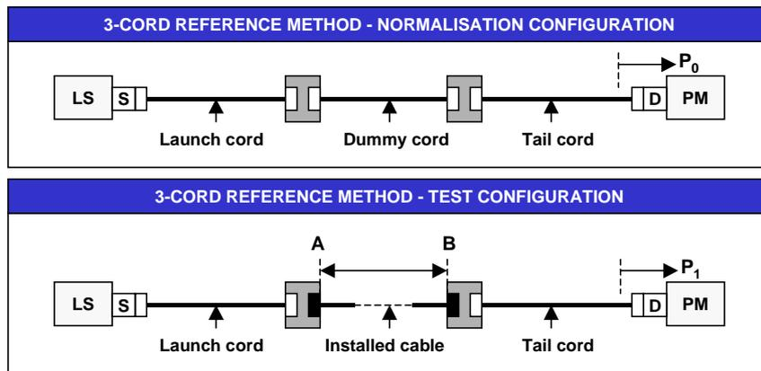
Figure 6 - 3-Cord Reference testing
