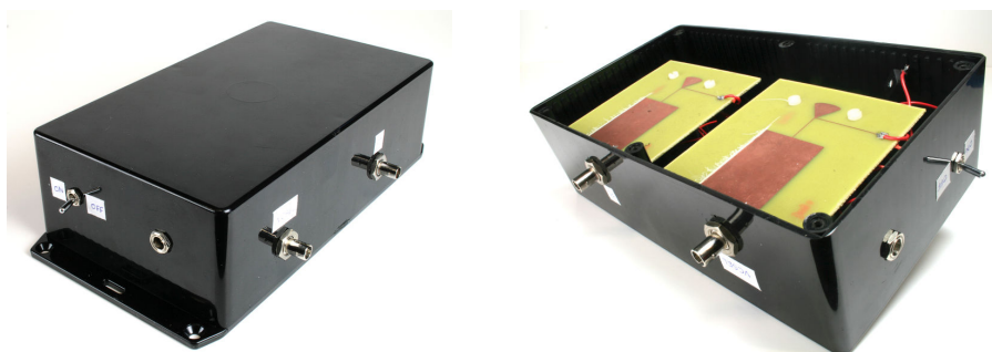
Figure 2 : Prototype PhAIA Module for use at the remote end of a WiFi range extension system
