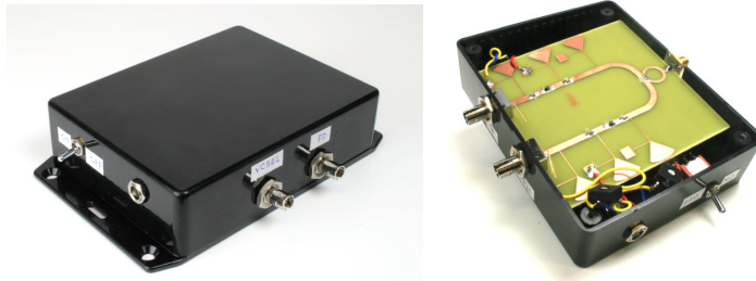
Figure 1 : Prototype Sampler Box for use in the WiPhAIA range extender system
