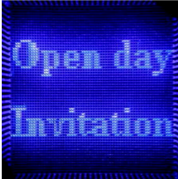
(This is a 64 x 64 element micro-LED array, actual size 2mm x 2mm)
